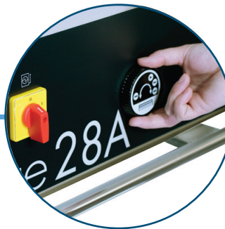
Electronic Back Gauge Adjustment Fine-tune control for precision cutting
